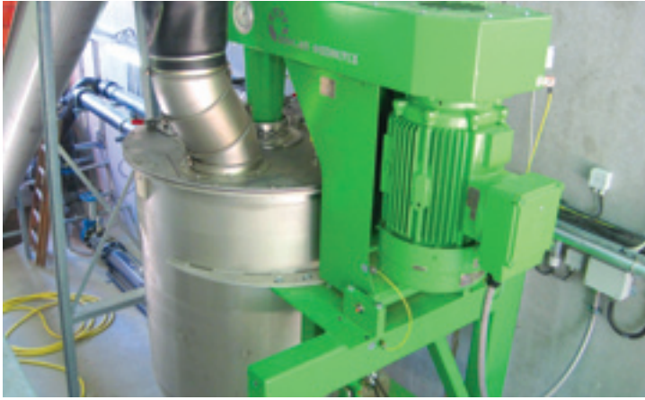
The Kreis-Dissolver greatly increases the gas output of a biogas plant.
